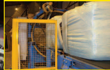
Guards protect operatives from moving parts on the SRF baling machine at the Northacre Resource Recovery Centre.
