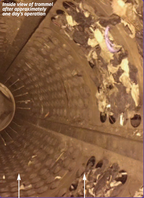
Area where metal tubes are yet to be fitted: Holes get clogged with waste and reduce efficiency
