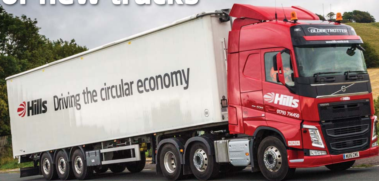
One of the new Volvo FH-500, 6x2 tractor units fitted with the Active Safety Package.
