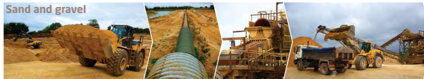
A 360° excavator breaks down the bank of aggregate whilst a loading shovel heads to the screener
