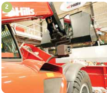
2 Manitou telehandler loads material onto a conveyor.
