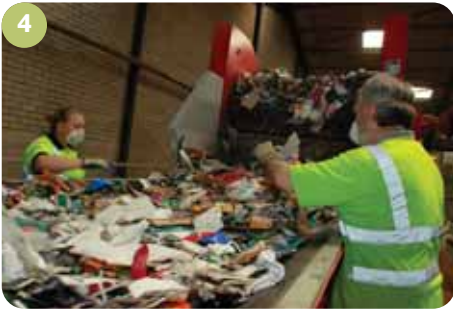
The material drops onto the first picking station, where operatives remove oversize and material such as plastic film, bags, buckets and non-plastic bottle/cardboard items.
