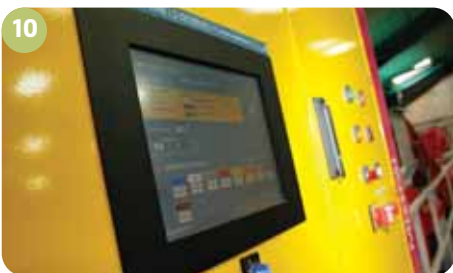
Inevitably, a small amount of material other than plastic bottles and cardboard is missed on the picking lines. The computer recognises many materials, including PVC, tetra pak, and polystyrene and makes a record of the number of objects of each material. This information can be used to improve sorting via the picking line or as a guide to adjust the optical separator to clean the residual material if required.
