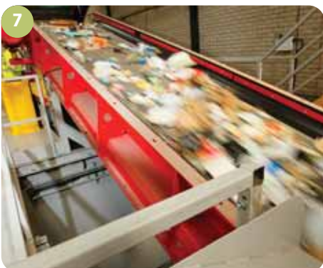
7 The undersize material from the OCC screen passes through a second picking line where waste material, for example coat hangers and CDs, and low quality plastic, such as trays and film, is removed.
