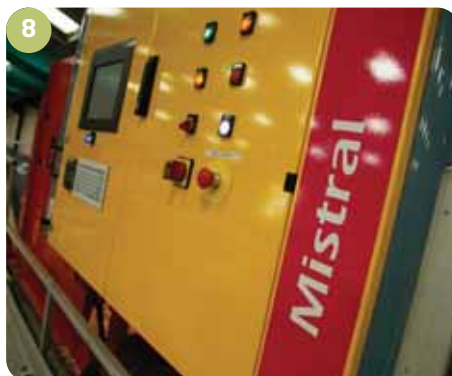
8 The optical separator, the final stage of the process, relies on Near Infra Red (NIR) technology. This super-fast, computerised technology can scan plastic material and determine its molecular structure.
