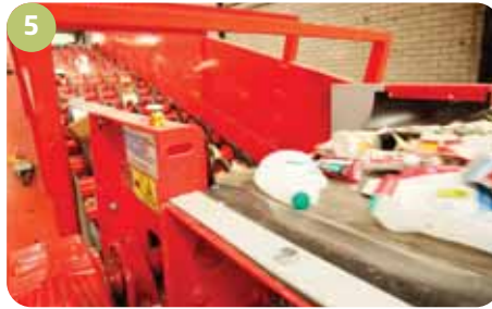
Remaining recycling material passes across the old corrugated cardboard (OCC) screen, which separates everything of A3 size or above. The remaining smaller material such as plastic bottles and small card falls through onto the undersize conveyor.
