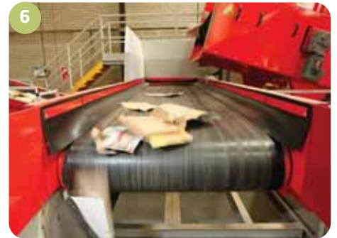
The large cardboard falls from the OCC screen onto a short quality control conveyor, and into a storage bay prior to being baled.
