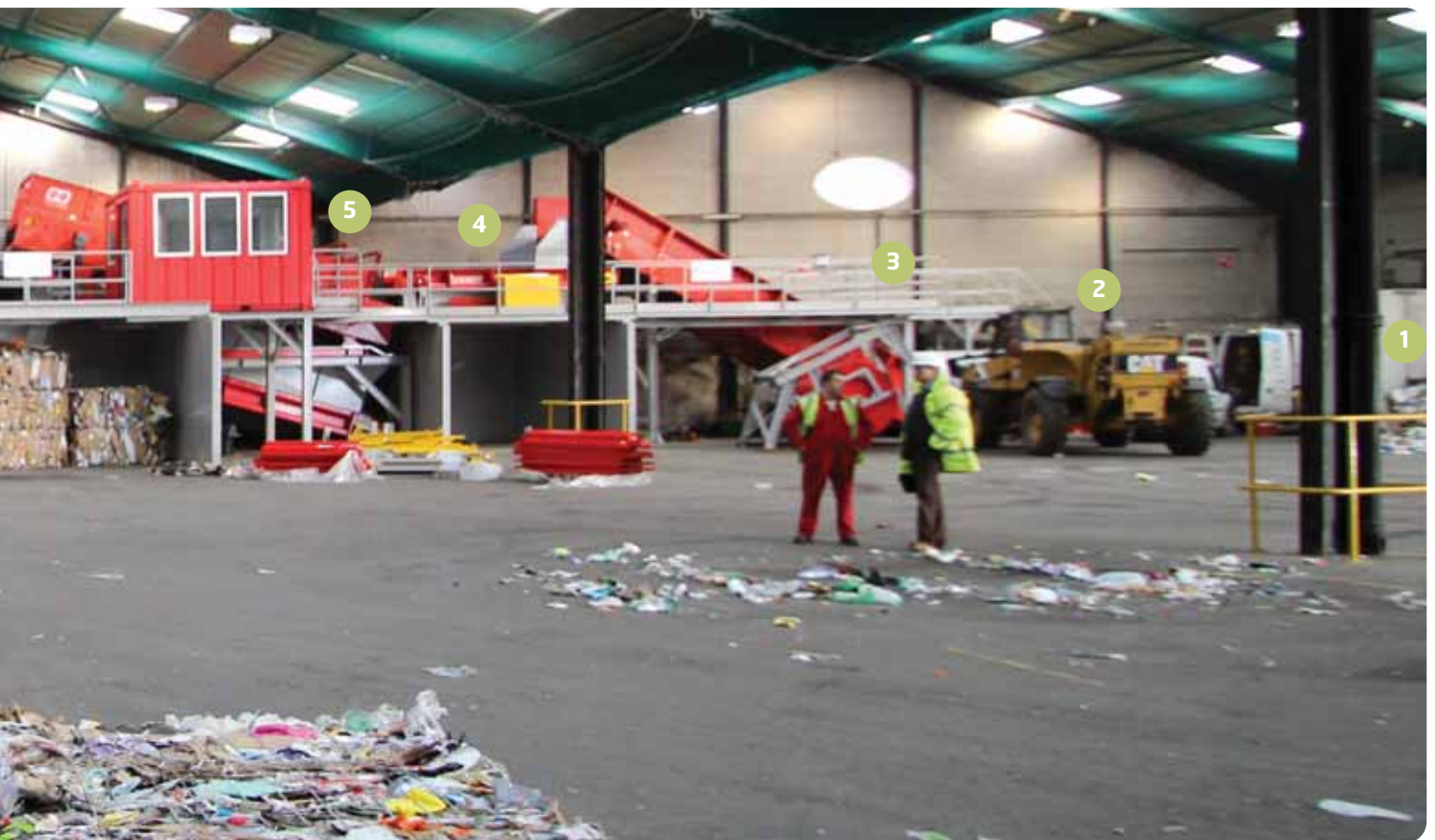
The material drops onto the first picking station, where operatives remove oversize and material such as plastic film, bags, buckets and non-plastic bottle/cardboard items.
