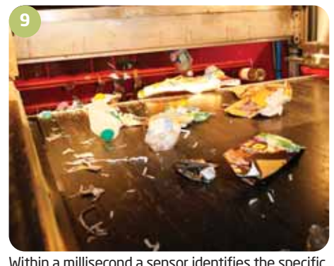
9 Within a millisecond a sensor identifies the specific type of plastic, and sends a signal to tiny air jets which 'shoot' the material off the conveyor into separate collection bays. The recycling material is separated into three bays; PET plastic, HDPE plastic, and the remaining cardboard material.
