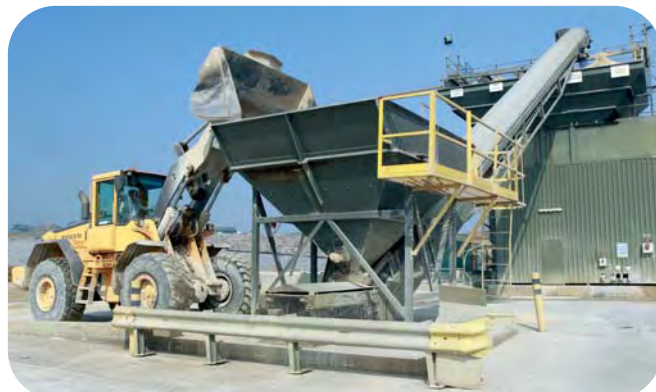
Jamie Woolford, mobile plant operative tipping materials into the ground hopper which feeds into the overhead storage bins
