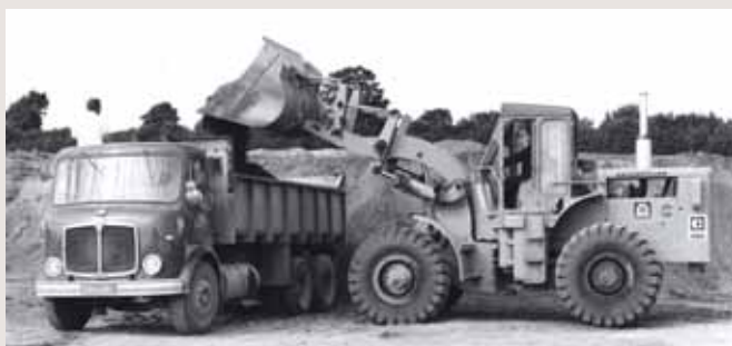
Using the dry digging method, a tractor shovel can dig and load in one operation
